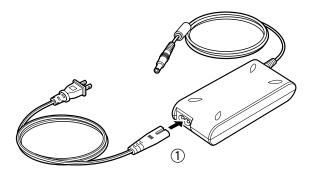
**2** Connect the AC adaptor power cord into the power connector ② on the rear of the scanner, and connect the power connect into a power outlet ③.
